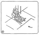
3 Then pull the thread clockwise 4 Slide the bobbin cover plate while pushing it down slightly over the bobbin. Allow about 4 inches of thread to show above the needle
